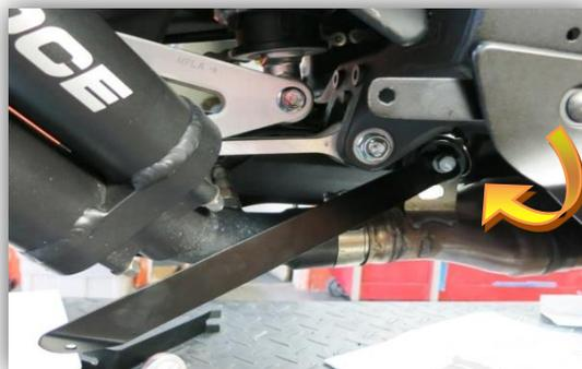
2. Install the forked end of the large bracket behind the 8mm exhaust bolt.
