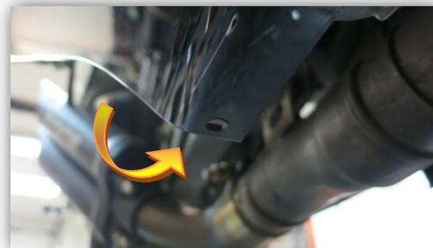
4. Once the shield is in position mark and drill a 6mm hole in the small lip on the bottom of the lower fairing.
