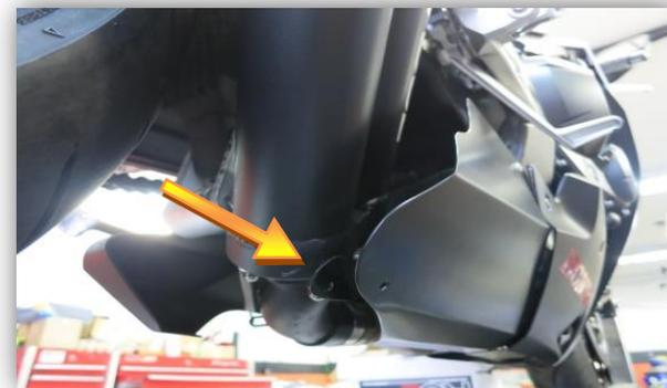
3. Install the shield using supplied hardware to the mounting brackets.
