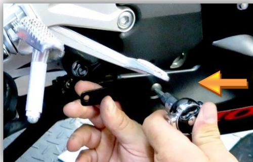
1. Install the small bracket behind the right fairing using stock fairing bolt.
