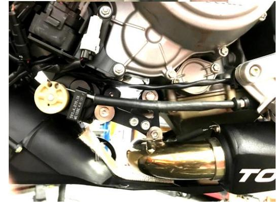
10. Install fairings and adjust shield worm gear clamp to fit as desired.
