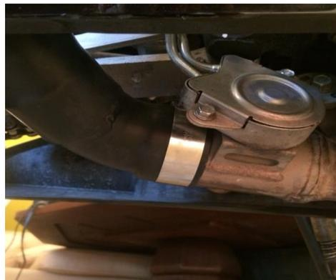
5. Attach your Toce T-Slash Exhaust System, align to ensure everything is lined up accordingly, and tighten all clamps from the header assembly back. You're finished!
