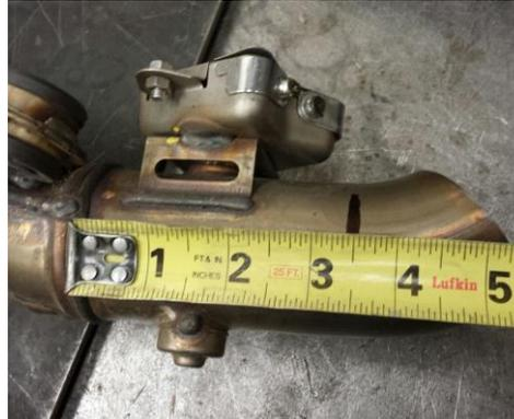
2. You need to cut the exhaust straight prior to the bend as you do not want any bends in your cut to optimize airflow.
