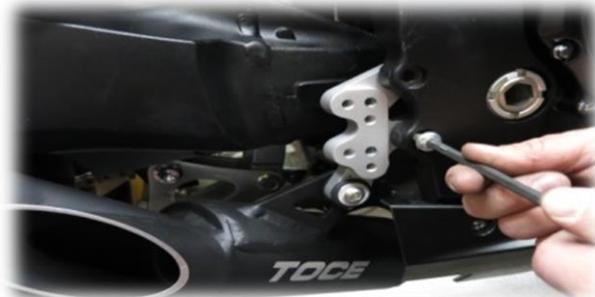
22. With exhaust installed adjust location of muffler and mid pipe so there is 1/2" to 3/4" gap between muffler and swing arm, then tighten the muffler bolt and T-bolt clamps.
