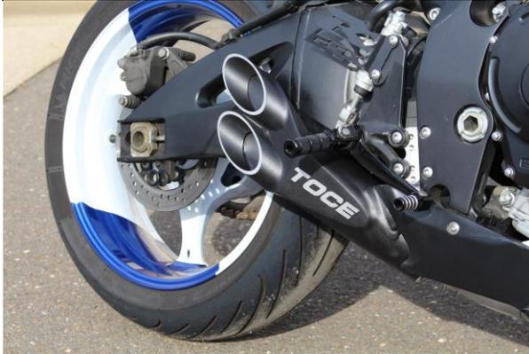
1. Remove right and left side fairing, and stock muffler.
