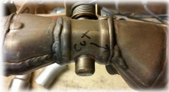
13. Sand or file off any sharp edges left by saw.
