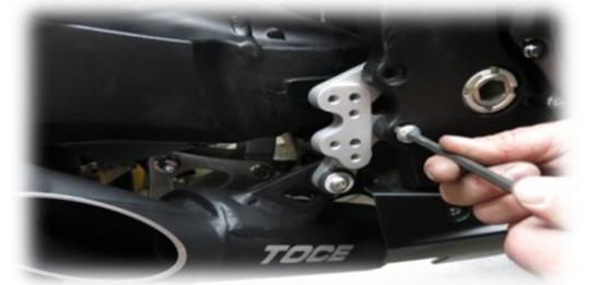
21. With exhaust installed adjust location of muffler and mid pipe so there is 1/2" to 3/4" gap between muffler and swing arm, then tighten the muffler bolt and T-bolt clamps.
