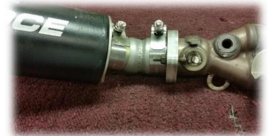
19. Rotate muffler and mid-pipe until the mounting bracket on the muffler lines up with the new foot peg adjuster plate mount.
