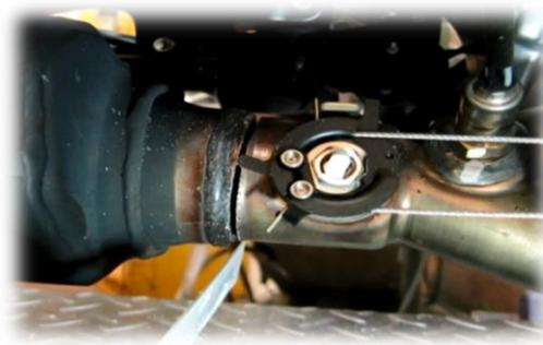
12. Cut exhaust with the provided Sawzall blade, behind exhaust valve (above)
