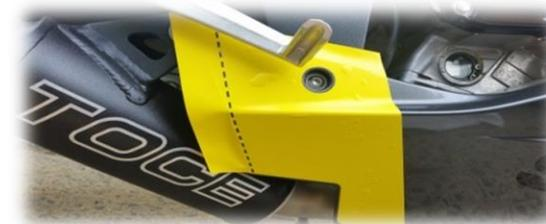
24. Using the cutoff wheel, cut fairing on dotted line. Remove decal
