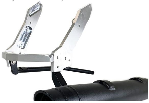
Note that the left bag support and the right side canister mount are affixed to the sub frame assembly from the inside and bolted from the inside. As shown. Reassemble and you're done!
