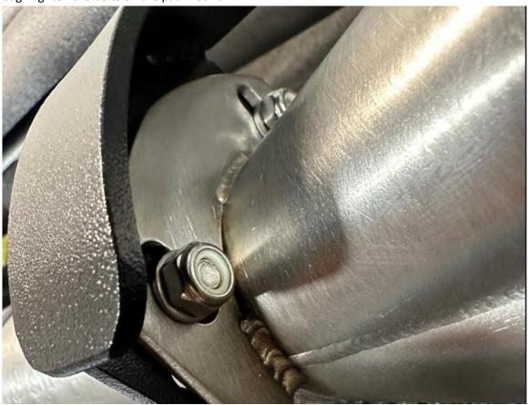
Note that the Capture bracket can help add additional height if needed. Ensure its positioning is allowing a smooth flow from heads to canister. There should not be any pressure of the system applying against itself.
