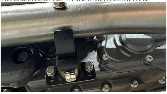
Install the canister assembly to the Y-pipe and affix to the factory mounting location on the subframe support. Install antenna mount if equipped/kept between mount and can.
