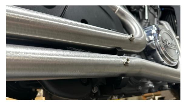
Proceed to tighten down tubes to the heads to factory specification. Onto the capture bracket's clamping bolt. The bolts to the block. Finally onto the canister bolts to the factory mount. At this point check the bag support and if in place well, tighten down the bag mounts. Mount the brake/foot rest back to the vehicle. If the unit wants to touch the exhaust, simply install the included black spacers between the frame and rest.
