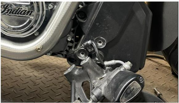
Proceed with loosening the header down tube bolts and oxygen sensors from each pipe. Unbolting the rest of the exhaust mount bolts, and remove the factory exhaust from the vehicle. Prep placing the Toce Exhaust into place by slightly loosening the capture bracket bolt pictured. This will allow for a bit of play for aligning the headers to the block.
